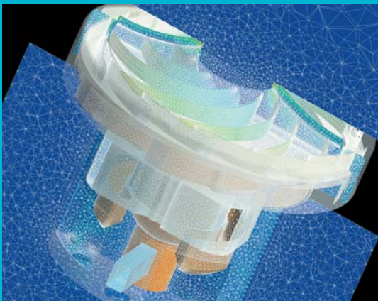
Grid generated with ANSYS ICEM CFD
