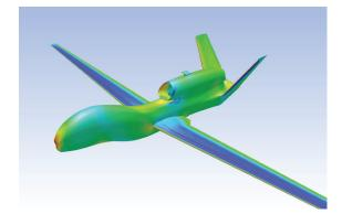
In this demonstration (and fictitious) example, ANSYS simulation software was used to improve the lift-to-drag ratio of a UAS wing over a range of angles of attack. Using goal-driven optimization, the geometry of the wing was automatically modified to achieve the desired improvement in lift. The result: a slightly modified platform that can deliver a much heavier payload.
