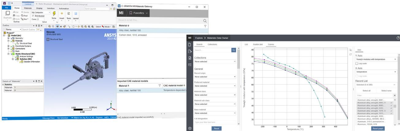
Figure 1. Comparison of materials using Ansys GRANTA MI Pro web application and assignment of materials in Workbench using the GRANTA MI Pro Workbench Gateway.
