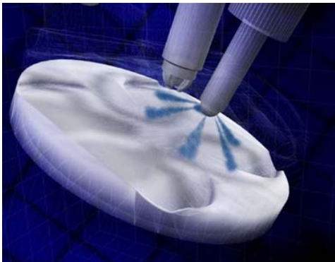
Figure 10: High-pressure direct injection hydrogen combustion engine. Courtesy BMW Group
