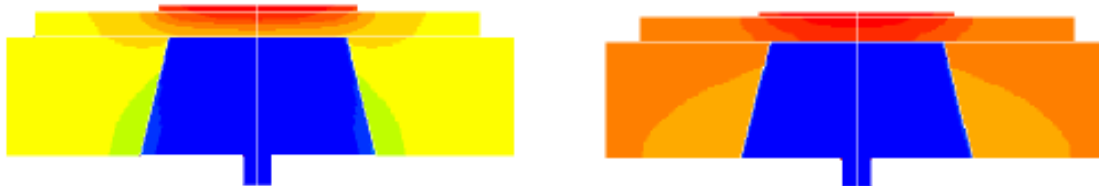
Figure 5: Temperature contours in IGBT package with boiling (left) and without boiling (right). 11
