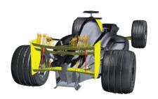
The adjoint solver indicates what portion of the geometry to modify and how to modify it to obtain the optimized down-force on this Formula One design.
