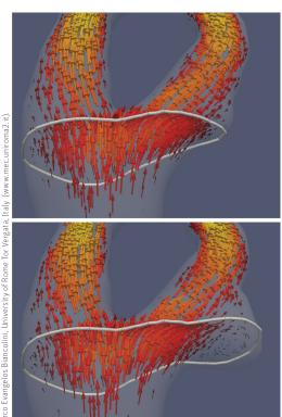
Thanks to the RBF-Morph solution, researchers can study different clinically relevant anatomical modifications of a carotid bifurcation. Morphing the computational grid to the different carotid bifurcation shapes dramatically speeds up the simulation process.
