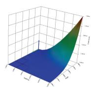
This response surface plot shows flow, arm angle and pressure loss data that can be used by engineers to optimize the design of the check valve shown in the above image. *Courtesy Cameron*.
