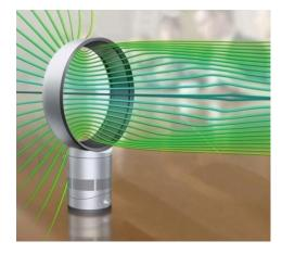
For the new bladeless fan, Dyson engineers developed a basic design concept in which air is drawn into the base of the unit by an impeller, accelerated through an annular aperture and then passed over an airfoil-shaped ramp that channels its direction.
