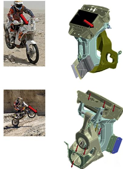
Figure 2. Exemplary samples of load cases for component design — maximum load impact upper body on roadbook (top), operating load while jumping (bottom).
