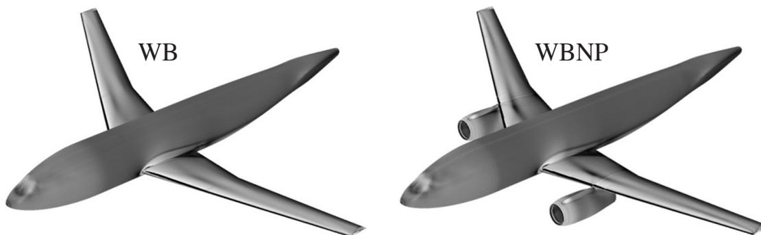
**Figure 4.** Geometries of DLR-F6 models for AIAA Drag Prediction Workshop (Courtesy DLR Braunschweig.)
