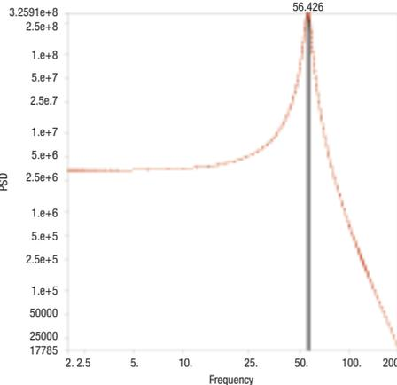
Figure 7. Response power spectral density of bending stress distribution for aluminum beam
