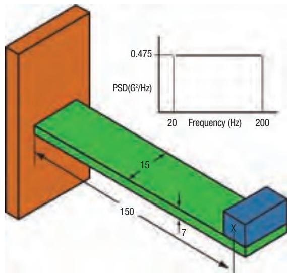
Figure 5. Problem sketch of aluminum beam with a weight at the tip undergoing white-noise random vibration
