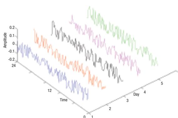
Figure 1. Random vibrations measured for vehicle on a rough road showing periodicity for single, dual and quad disk configuration
