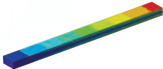
Figure 6. 1-σ bending stress distribution
