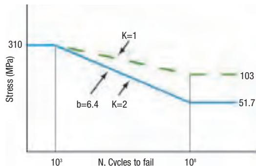
Figure 8. S-N curve for 6061-T6 aluminum beam with a stress concentration of 2
