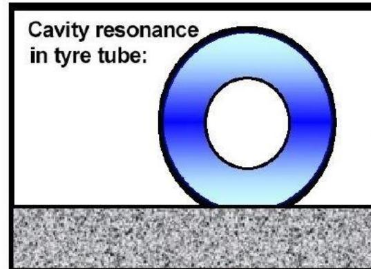
Acoustic resonance in the air space inside the tire
