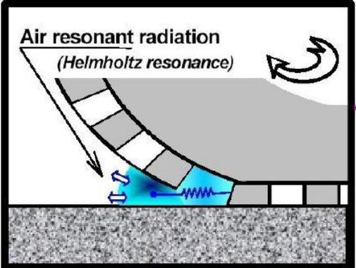
Sound amplification caused by organ pipe and Helmholtz resonator geometries within the contact path
