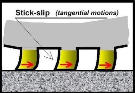
Slip-stick motion of the tread block on pavement
