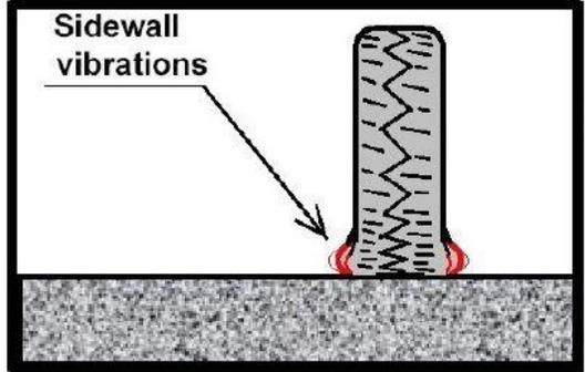
Vibration of the tire carcass around the tread band and at the sidewall of the contact patch
