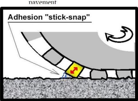
Adhesion between the tread block and pavement at the exit of the contact patch
