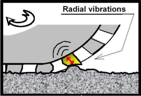
Vibration caused by tread block/pavement impact
