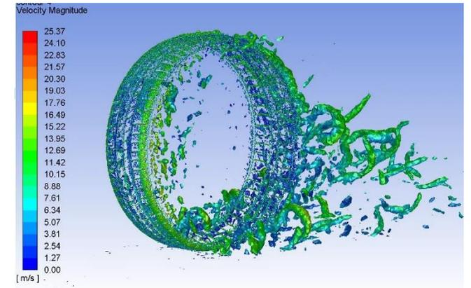
Velocity Contours on Iso-surfaces (Q criterion)
