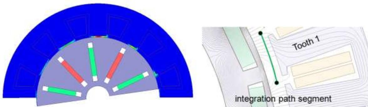
Fig. 3: Co-energy distribution inside the air gap and stator of a synchronous machine with permanent magnets and reduced force integration path
