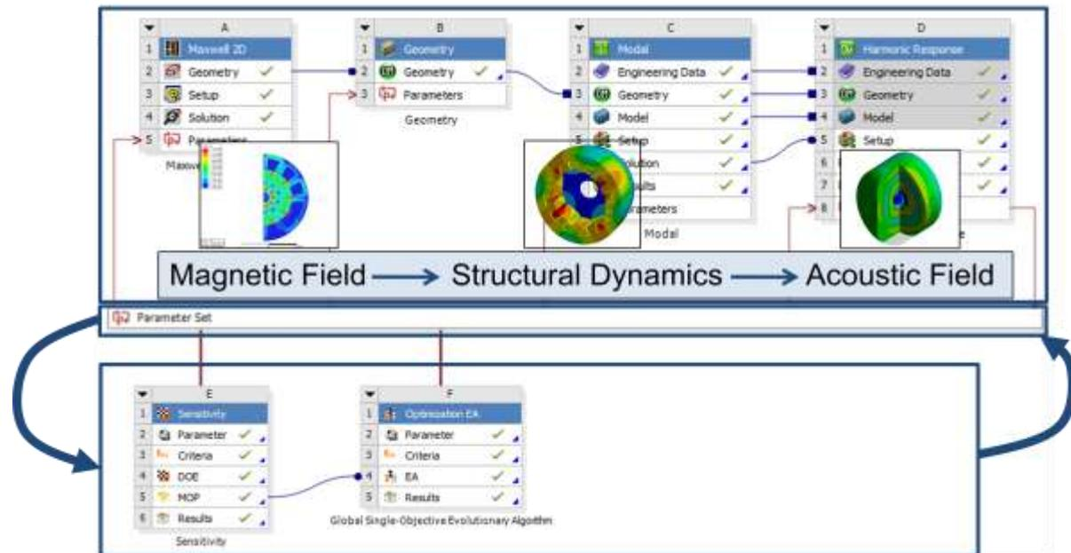
Fig. 4: Full parameterized optimization environment in ANSYS Workbench
