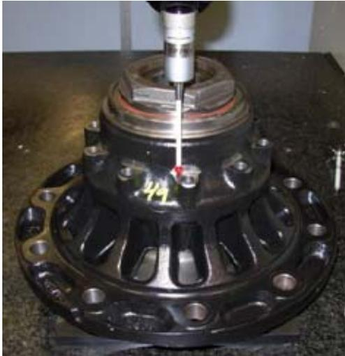
To verify the results of the numerical simulation in terms of the mean value and scatter, 250 assemblies were measured as showed in Figure 9. The measurements results showed in Figure 10 indicate that there is good correlation with the numerical simulation results.
