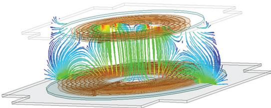
Figure 1. Flux lines calculated with ANSYS Maxwell
