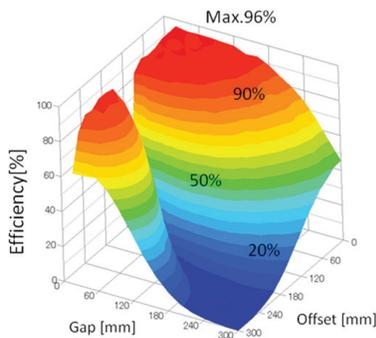
Figure 4. Efficiency map for power transmission system considering axial offset and gap
