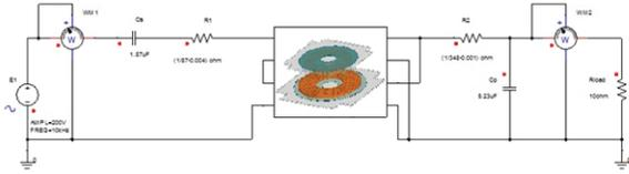
Figure 2. ANSYS Simplorer schematic of a simple power transfer system, cosimulating with transmitter and receiver coils from ANSYS Maxwell
