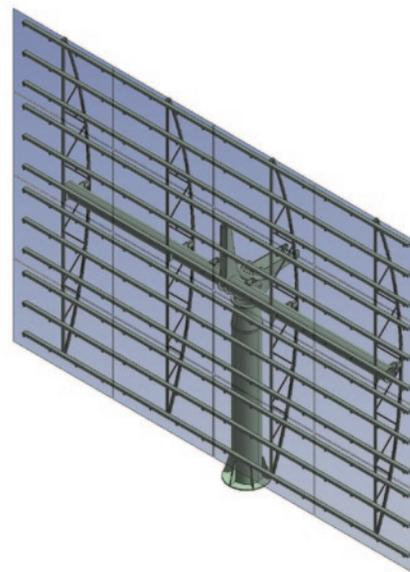
▲ Finite element model of heliostat created in ANSYS DesignModeler
