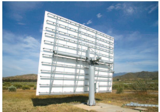
▲ NEM heliostat prototype
