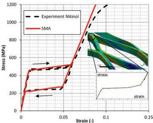
▲ Stress prediction for selected point on the stent helps determine fatigue life of stent.
