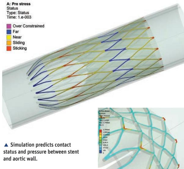
simple to unite fluid and structural models in a two-way coupled transient simulation using system coupling. The transient fluid-structure interaction simulation was run from 0 to 0.3 seconds.
