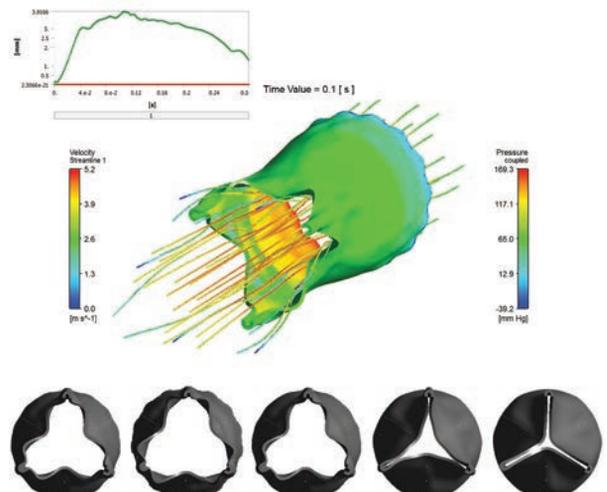
▲ Deformation of stent due to blood flow as predicted by multiphysics simulation
