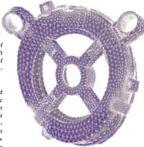
Using the design optimization capabilities of ANSYS, WEG conducted a finite element analysis of the optimized geometry of DE and NDE aluminum endshields used in washing machines.
