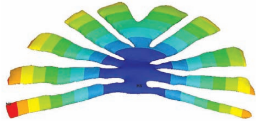
Structural analysis results show load required to deflect bone and deformation of the forehead bone after deflection.
