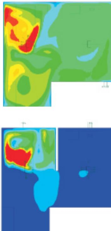
Contaminant concentration contours, at an elevation of 1.4 m above the floor originating from patient 1. The figure on the top has no partition, while the figure on the bottom uses a partition and ventilation systems local to each patient.
