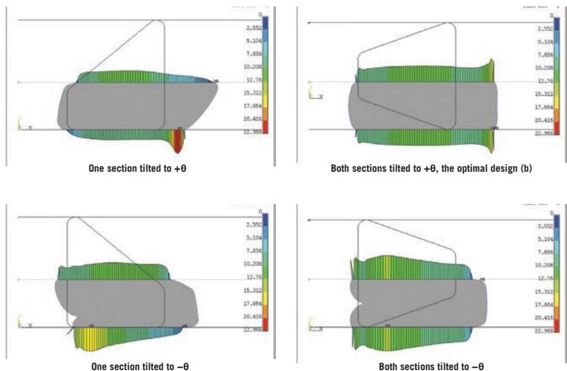
▲ Distribution of seal surface pressure after 200,000 hours for gasket with tilt angle ( $\theta$ ) of 40 degrees
