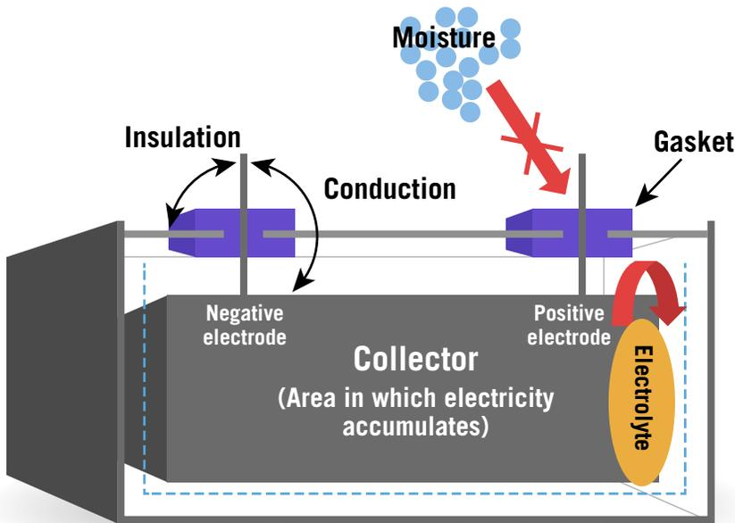
▲ Diagram of Li-ion battery showing gaskets
