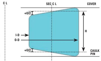
▲ Cross-sectional shape of circular gasket with axial symmetry when both upper and lower sections are tilted in relation to horizontal plane
