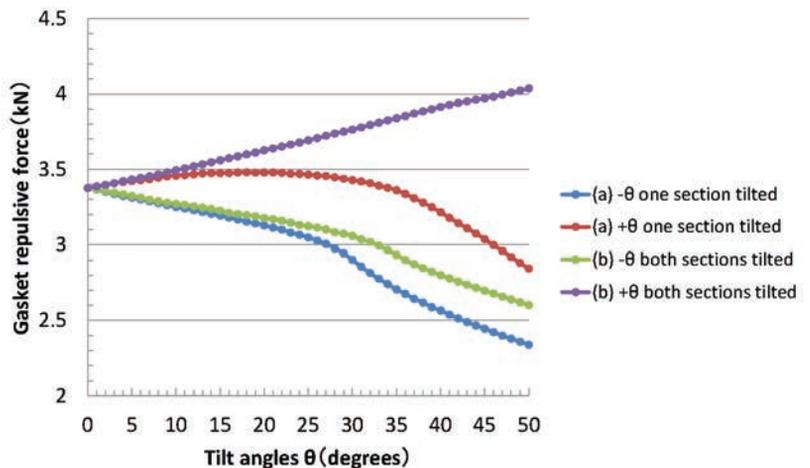
▲ Changes in gasket repulsive force after 200,000 hours with one or two sections tilted and different tilt angles
