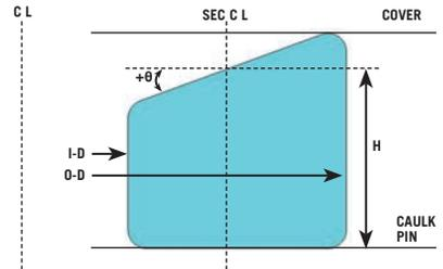
▲ Cross-sectional shape of circular gasket with axial symmetry when upper section is tilted in relation to horizontal plane
