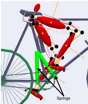
Figure 1. Two springs suspended between the frame and the crank mechanism. The two green "cylinders" indicate the position of two similar springs.
